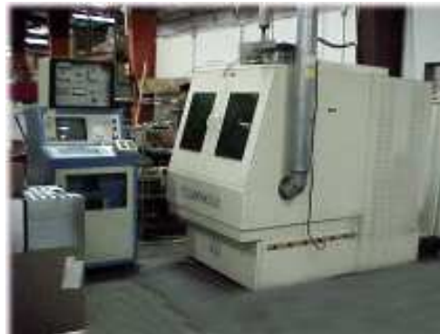
YAG laser welder 400w Lumonics System 2000
